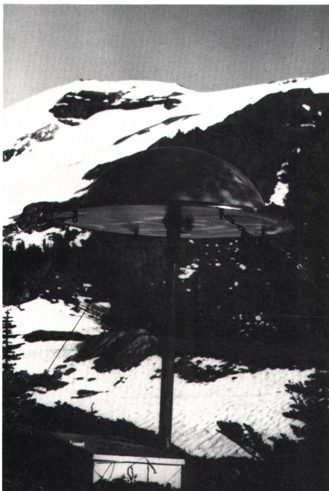
FIGURE 73.—Data collection platform, Mount Baker, Wash. The diameter of the Plexiglas-covered antenna is 1.2 m.
