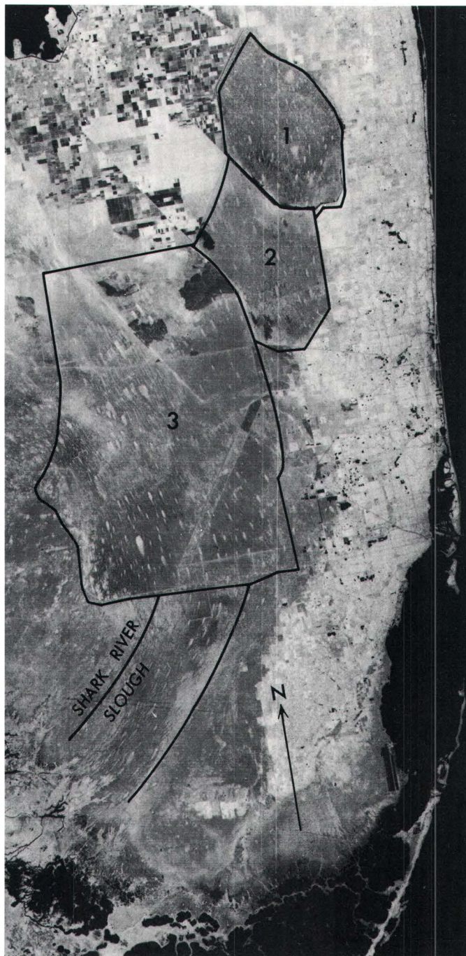
FIGURE 114.—Determination of surface-water storage in Conservation Area No. 1. Schematic diagram of the use of space-relayed data to calculate surface-water storage. ERTS data from three successive passes on Feb. 14, Mar. 4, and Mar. 22, 1973, of Conservation Area No. 1 are used to demonstrate the feasibility of determining surface-water storage.
