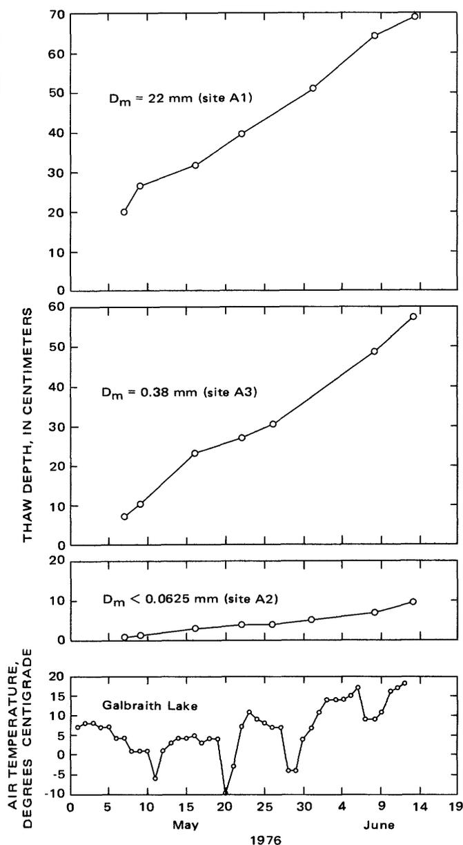
FIGURE 4.—Thaw depths in emersed bed and bank material of differing texture at three sites on the Atigun River. Air temperature was measured at Galbraith Lake.
