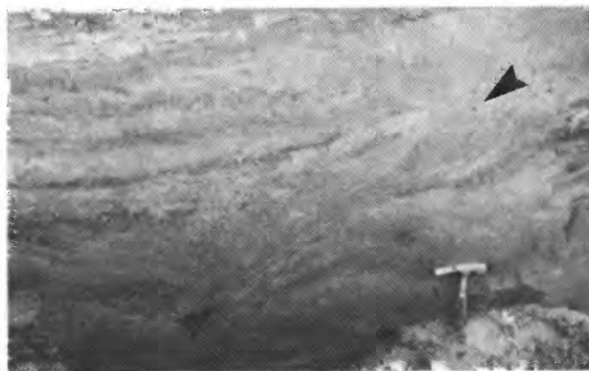
FIGURE 8. — Photograph of 0.5-m-wide fault zone (between arrows) exposed in USGS exploratory trench located at base of Reelfoot scarp. Faults displace alluvium in a normal sense and may be continuous with the subsurface Reelfoot fault. Location of trench shown on figure 1.
