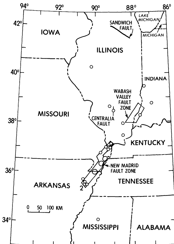
FIGURE 2. — Epicenters of damaging earthquakes in the central Mississippi valley. Large circles refer to epicenters of the three major earthquakes of 1811-12. Epicenters of the 203 damaging aftershocks are not plotted. Small circles refer to damaging earthquakes subsequent to 1812. The number 2 indicates two earthquakes with the same epicenter.
