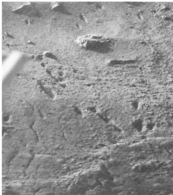
FIGURE 57.—Impact craters and pits in drift material produced by fragments propelled by engine-exhaust gases during landing. Note low to nonexistent rims of craters and pits and small fragments in craters and pits as well as on surface. Alignments and elongations of craters and pits are radial to engines 1 and 2 (frame 11A022/004). Rock in top center of photograph is approximately 8 cm wide.
