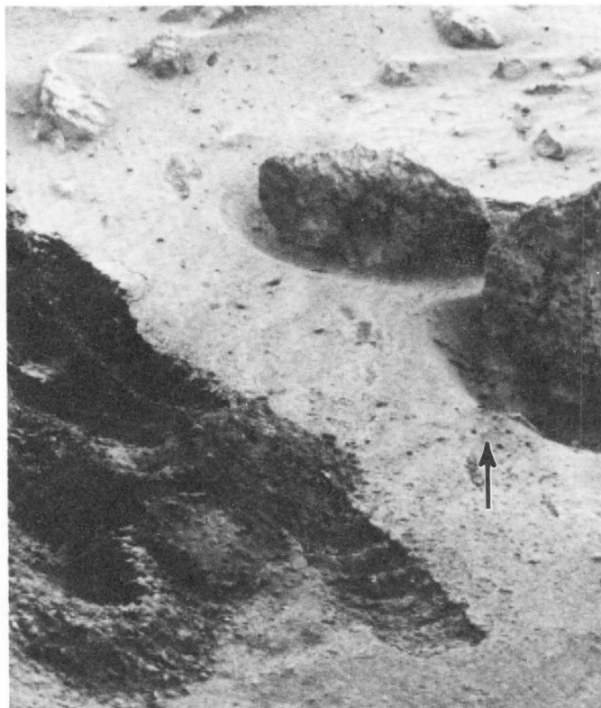
FIGURE 63.—Results of Sol 350 impact experiment on Mars, Lander 1. Largest fragment (arrow) is about 0.45 cm wide but others are about 0.3 cm to below resolution of pictures (0.15 cm). Fragments appear to have penetrated \frac{1}{2} or less of their diameters. Pretest surface shown in figure 62. Free-fall velocities were about 2.5 m/s (frame 11E082/351).
