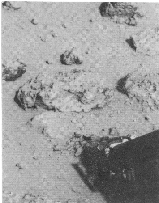
FIGURE 79.—Collector head of Lander 2 inserted in crusty to cloddy material during diurnal temperature measurements. Shadow of camera 2 is cast along azimuth of boom and collector head (frame 21E236/405). Large rock (rock 14) in center of picture, just beyond collector head, is about 22 cm wide.
