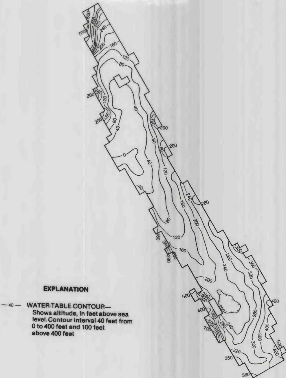
FIGURE 14B.—Predevelopment water-table altitude.
