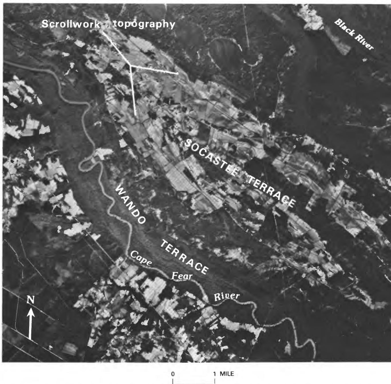
FIGURE 9.—Aerial photograph of the lower Cape Fear River valley. Upland sediments (Waccamaw and Penholoway Formations) lie southwest of the Cape Fear River, and valley sediments lie to the northeast. Just upriver from the confluence of the Cape Fear and Black Rivers, elongate areas of Carolina bay-covered Socastee terrace are surrounded by scrollwork topography characteristic of the Wando terrace.
