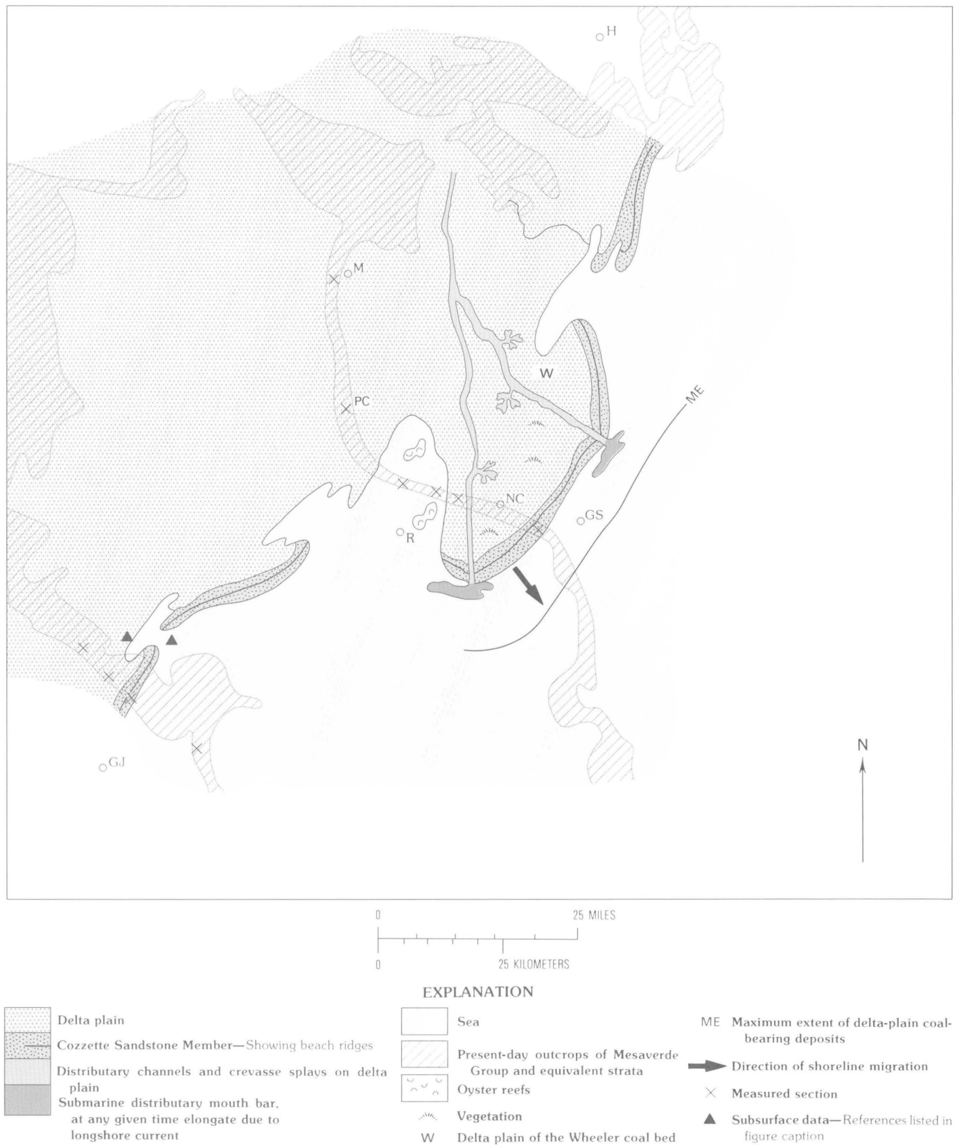
FIGURE 20.—Schematic sketch of coastal paleogeography during deposition of the Cozzette Sandstone Member and the Wheeler coal bed, before or during the time represented by range zone of E. jenneyi , based on data from Grand Hogback (this report; Collins, 1976; Gill
