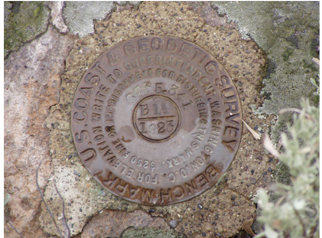
Close up of bench mark.
