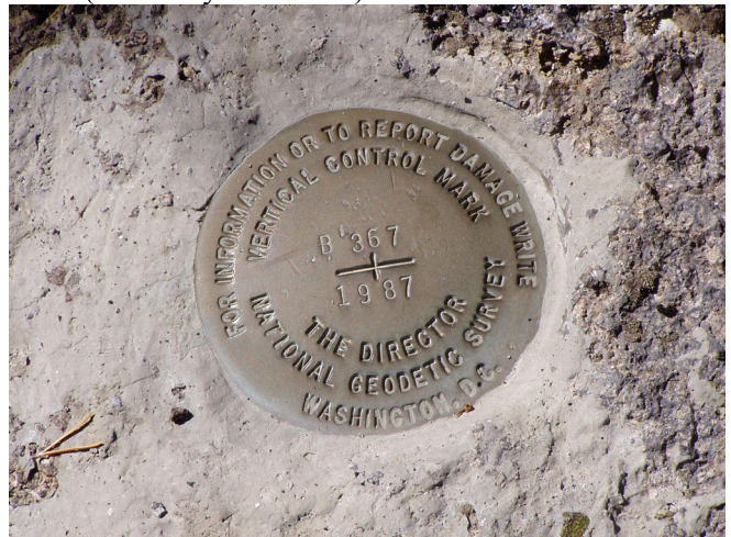
Close up of bench mark.
