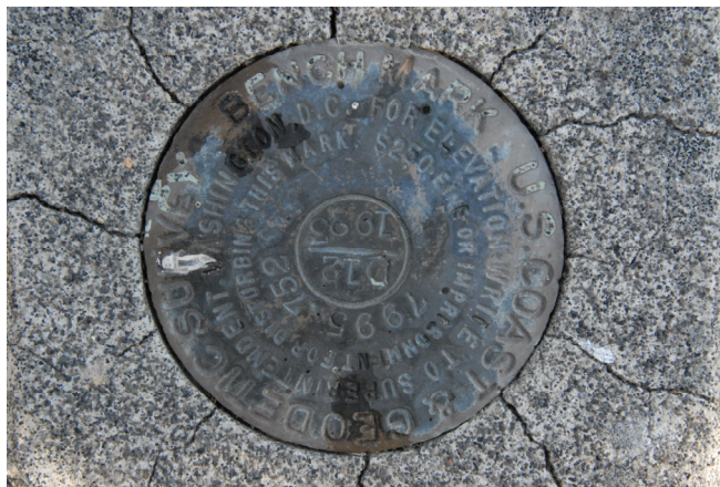
Close up of bench mark.
