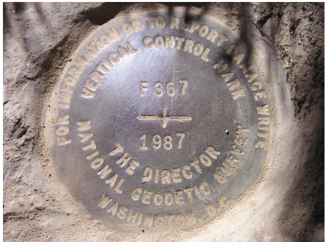
Close up of bench mark.
