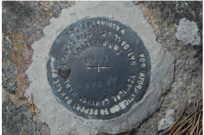
Close up of bench mark.
