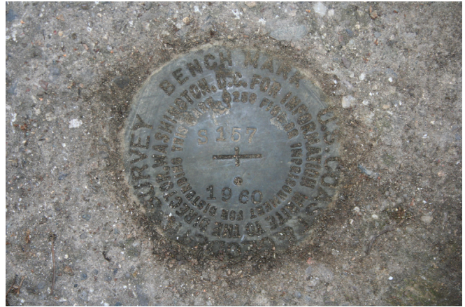
Close up of bench mark.
