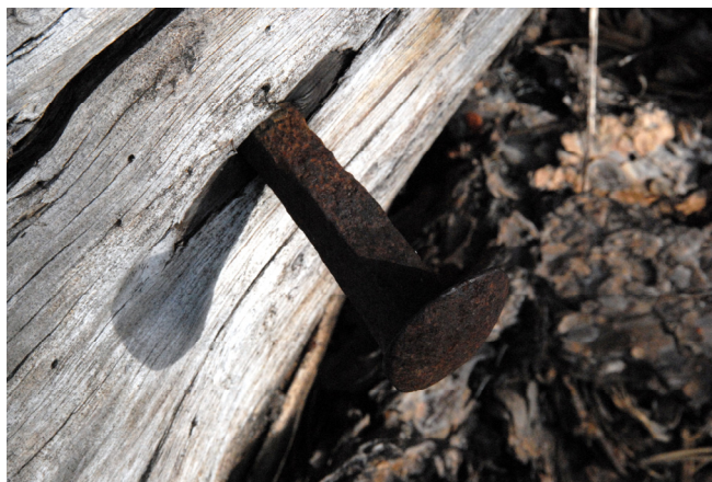
Close up of bench mark.
