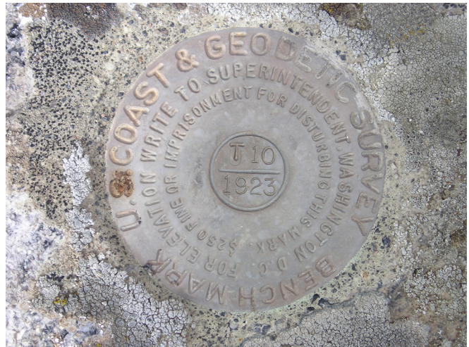
Close up of bench mark.
