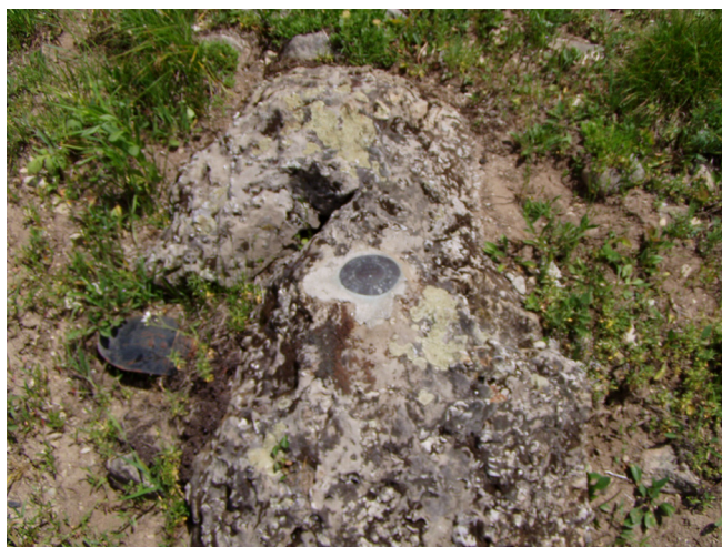
Close-up of bench mark.
