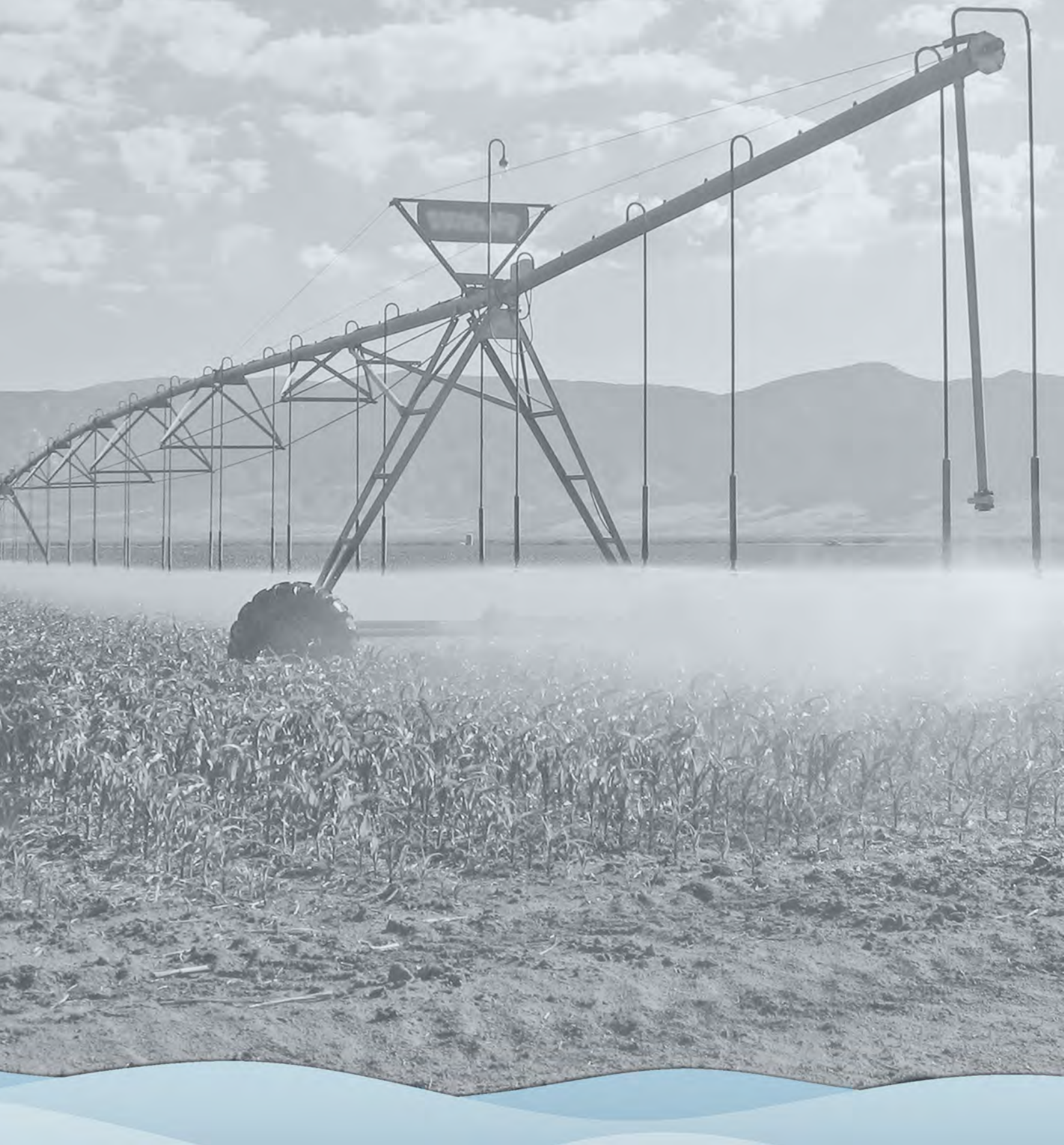
Typical, large-scale center-pivot spray irrigation system. Photograph by U.S. Geological Survey.
