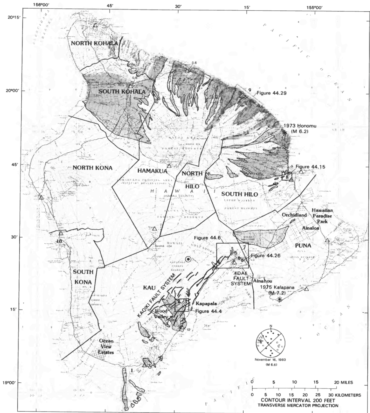
FIGURE 44.1.—The Island of Hawaii showing epicenters of November 16, 1983, Kaoiki earthquake and two earlier damaging earthquakes; also shown are areas of 1983 structural damage and earthquake-related ground failures discussed in text. Additional text figures cited where applicable. Inset shows focal-mechanism solution for 1983 earthquake from Endo (1985, p. 186): P -wave first motions plotted on lower hemisphere equal-angle stereonet; open squares, down first motions; solid squares, up first motions. Topography from U.S. Geological Survey Hawaii Island series W532, 1975, 1:250,000.
