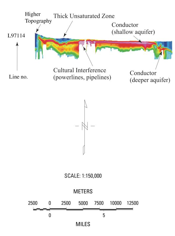
Conductivity vs. Depth Fence Diagram Superimposed on a Topographic Map of the Fort Huachuca Area, Arizona
