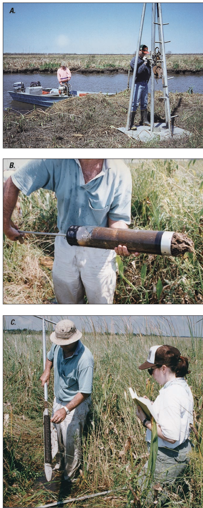
Figure 8. Marsh samplers, Bayou Perot intermediate-marsh sample locality—(A) vibracore equipment; (B) Hargis sampler, and (C) McCauley peat borer (Russian peat borer).
