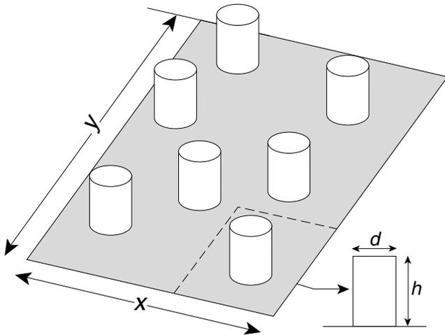
**Figure 1.** Schematic drawing of an array of roughness elements, illustrating dimensions used in calculation of lateral cover (adapted from Marshall, 1971). In this example, ground area  $S = xy$  is occupied by  $n = 7$  cylindrical roughness elements, each with frontal area  $F = hd$ . Lateral cover is given by equation 1.
