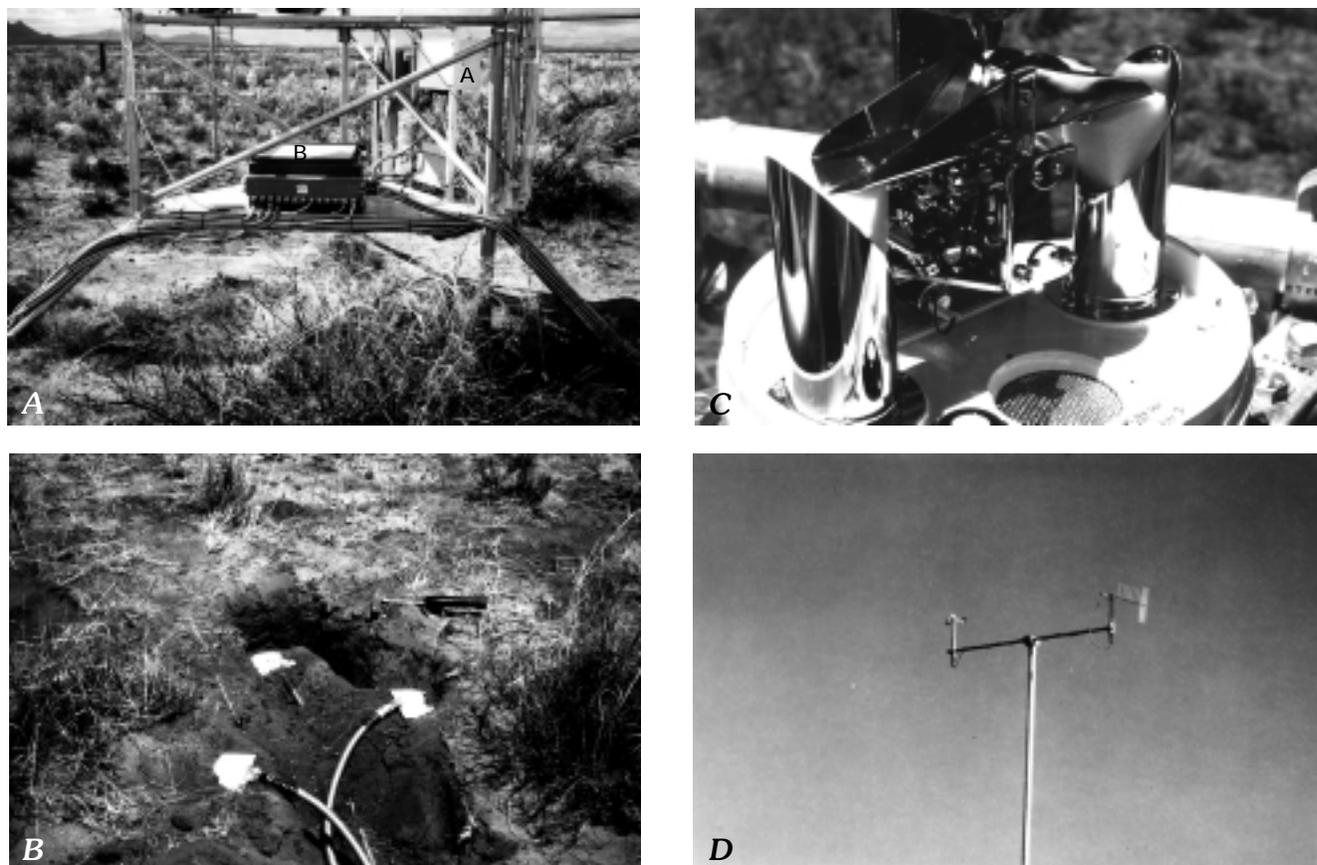
**Figure 4.** Close-up views of some components of Geomet stations. *A*, A close-up view of DCP tower at Jornada showing two different DCP's: shown at *A* is Model 540 Handar DCP; shown at *B* is environmentally sealed enclosure box for model 570 Handar DCP, which requires special protection from elements. *B*, Heat-flux sensors with buried cables; *C*, Open precipitation gauge showing tipping bucket; *D*, Wind-direction vane with needles.
