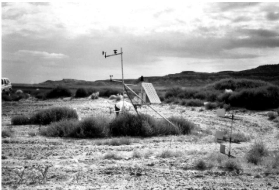
**Figure 10.** Automated DCP ministration (left) and windblown-particle catcher (right) monitoring wind erosion on field near village of Kyokotsmovi (New Oraibi) on Hopi Indian Reservation, north-eastern Arizona (Helm and Breed, chap. B, this volume).
