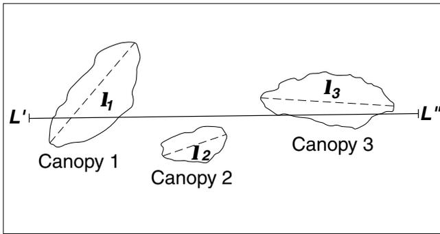
**Figure 5.** Schematic plan view of portion of line transect ( $L'$  to  $L''$ ) illustrating criterion for inclusion of plant canopy in sample obtained by line intersect sampling (LIS). Each canopy has unique "needle,"  $I_i$ , defined as long axis of imaginary envelope surrounding canopy. Canopy is included in sample if and only if "needle" is intersected by transect line; only canopy 1 meets this requirement in this example. (From de Vries, 1979.)
