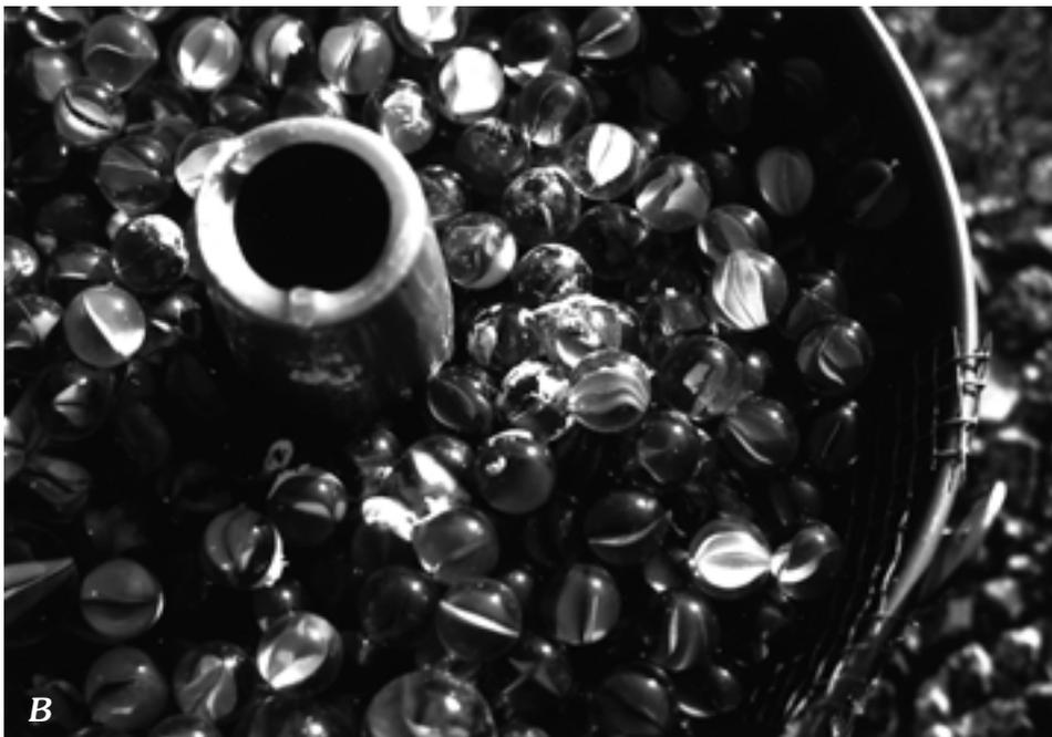
**Figure 2.** Photographs of dust-trap equipment. *A*, dust trap consisting of angel-food cake pan mounted on steel fence post 2 m above ground. Bird defenses (crossed metal straps coated with Tanglefoot) arch above the pan. Four sites in the network also have duplicate dust traps enclosed within a wind baffle, shown here with access gate open. *B*, closeup of marbles in pan resting on galvanized hardware cloth; white splotches are bird feces.
