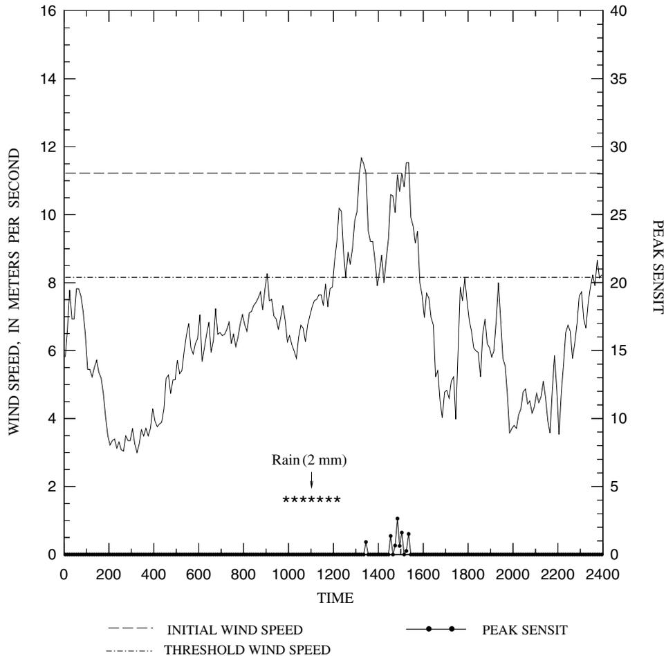
**Figure 13.** A spring storm at Yuma (March 1, 1991) showing a 2-mm rainfall at the beginning of the storm and sand moving, as recorded by the SENSIT, 1 hour later.
