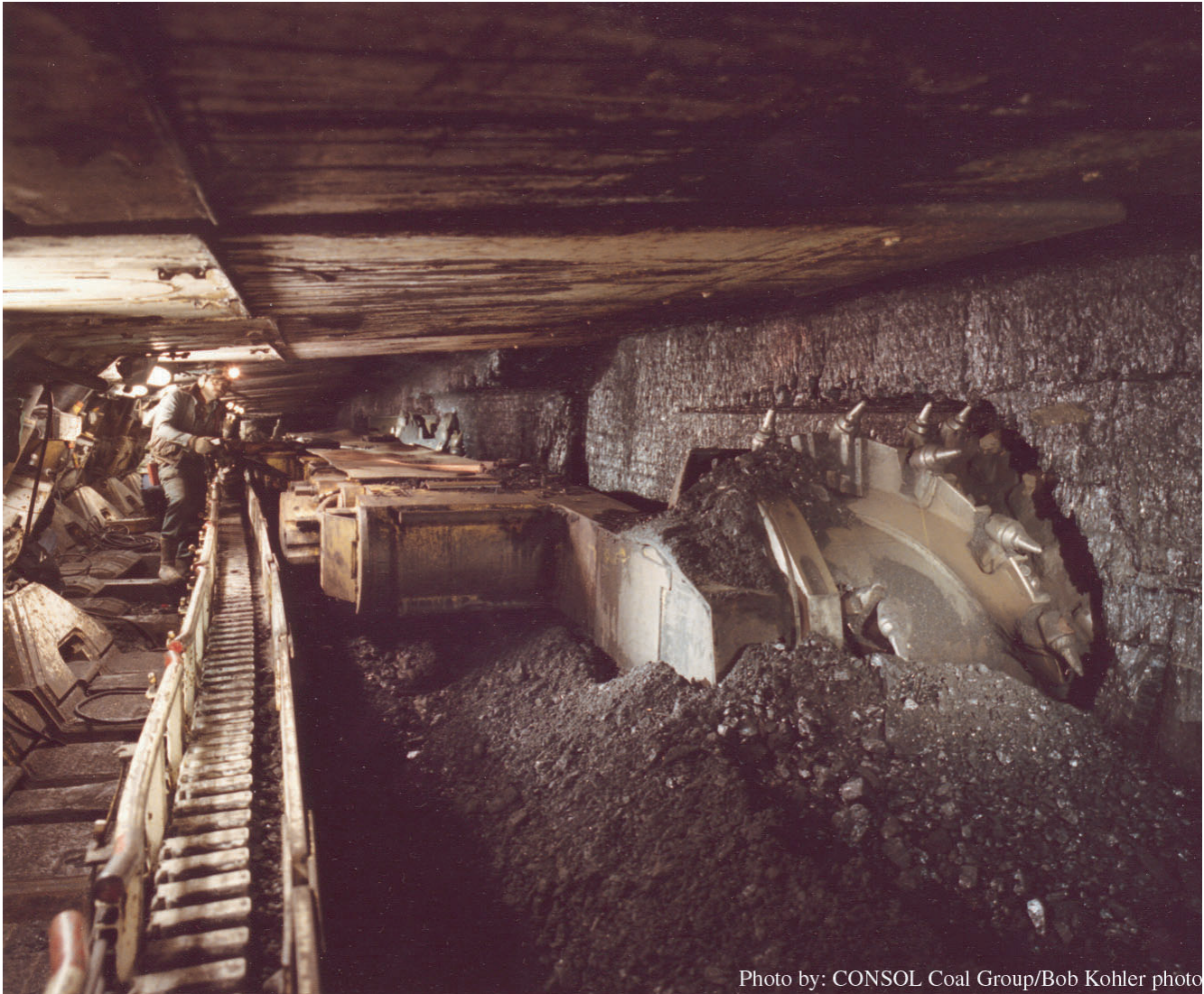
Figure 14. Photograph showing longwall mining operation in the Pittsburgh coal bed of the Monongahela Group in northern West Virginia. Photograph by CONSOL Coal Group/Bob Kohler Photography.
