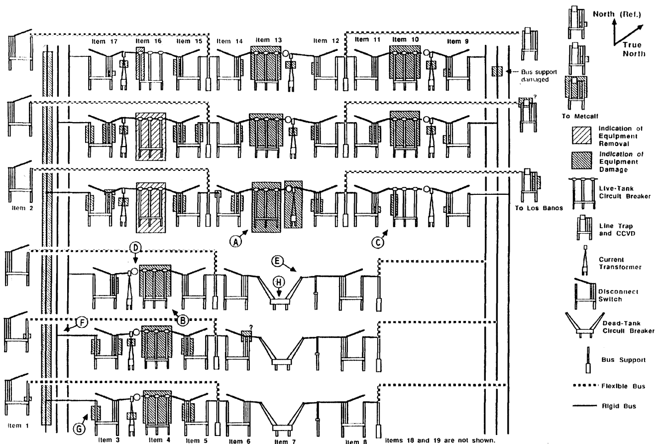
Figure 3.—Schematic diagram of 500-kV switchyard at the Moss Landing Substation (fig. 1), showing locations of damaged and removed equipment and numbered items referred to in text. Equipment shown as undamaged may have required repair that was not obvious from cursory inspection. A, 500-kV circuit breaker (fig. 6); B, interrupter heads on 500-kV live-tank circuit breaker (fig. 7); C, interrupter-head-support columns on 500-kV circuit breaker (fig. 8); D, 500-kV current transformer (fig. 9); E, support of 500-kV current transformer (fig. 10); F, disconnect switch with rigid bus (fig. 11); G, disconnect switch with flexible bus (fig. 12); H, disconnect switch of channel design (fig. 13). CCVT, capacitatively coupled voltage transformer.
