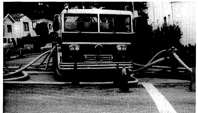
Figure 3.—San Francisco Water Department pumper providing booster-pump services to supply areas that were out of water because of numerous earthquake-related water-main breaks.
