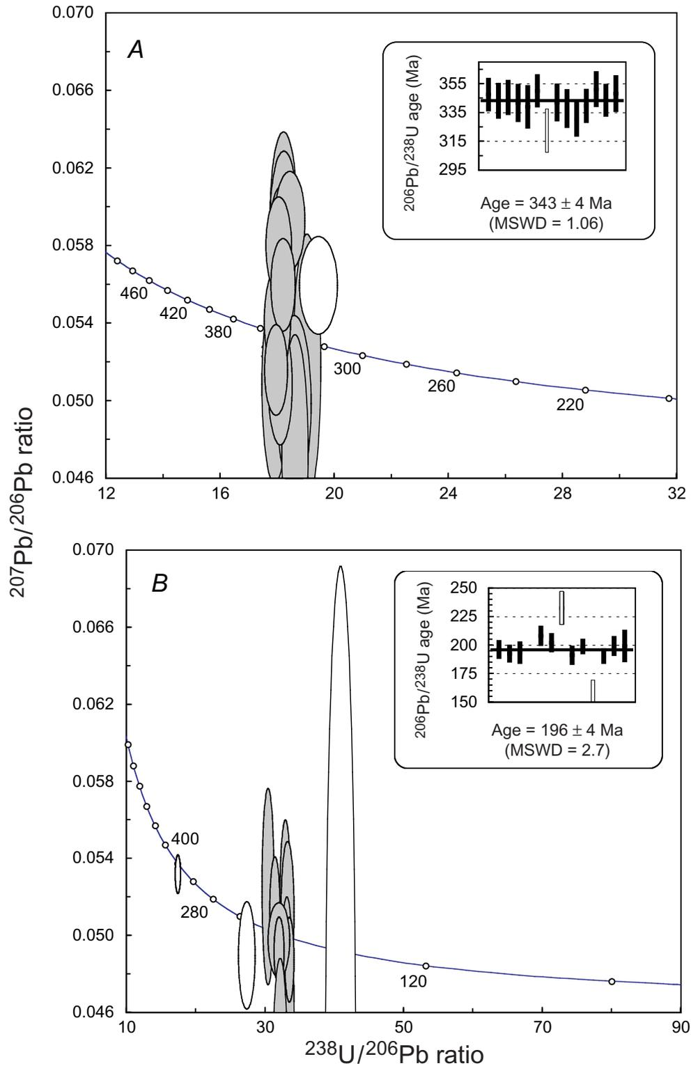
**Figure 6.** Tera-Wasserburg plots of U-Pb-isotopic data for zircons from the Fortymile River area, east-central Alaska. *A*, Sample 98AD174 (table 1). *B*, Sample 98AD296 (table 1). Error ellipses,  $1\sigma$ ; weighted average error bars,  $2\sigma$ . Filled error bars, corresponding to filled error ellipses, were used in weighted-average calculations. MSWD, mean square of weighted deviates.
