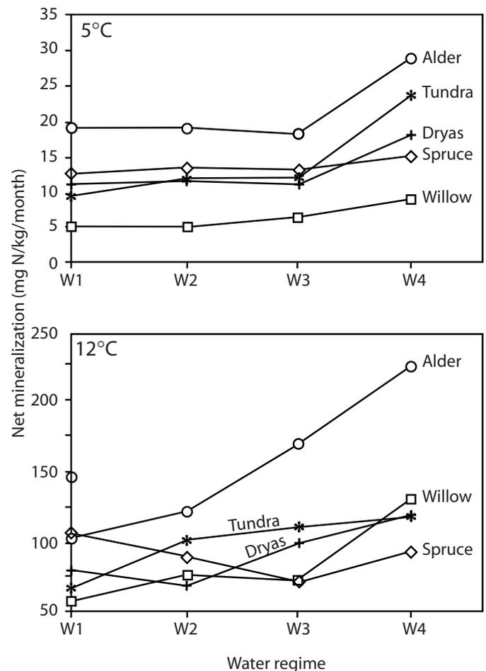
**Figure 4.** Laboratory net N mineralization in response to changes in temperature (5 and 12°C) and moisture. Responses to moisture and temperature were significant ( $p < 0.05$ ). Water treatments: W1, one moisture addition at beginning of 30-day incubation; W2, two moisture additions or two wet/dry periods; W3, three wet/dry treatments; W4, four wet/dry treatments. From Binkley and others (1994).
