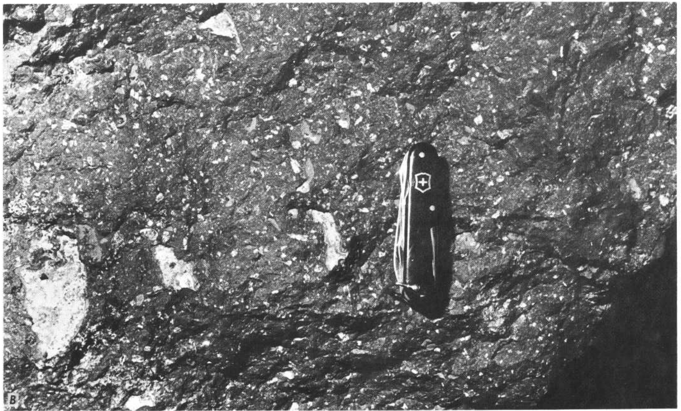
A CLOSER LOOK AT BASALT. A, Piece of dense basalt, natural size. B, Basalt that has many bubble holes, now filled by calcite and zeolite; half size. C, Slice of basalt, magnified 8 times. Large crystals of olivine with corroded edges (upper left) "floating" in a mixture of glass (dark gray) and tiny crystals of feldspar, pyroxene, and olivine. Large black area is a hole where a crystal was pulled out of the rock slice during grinding. Doubly polarized light. (Fig. 47)
