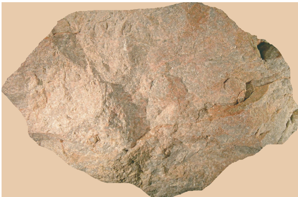
Figure 8. Fine-grained massive quartz-alunite replacement (mapped as unit qap of acid sulfate suite) of altered lavas or volcaniclastics of Silverton Volcanic Series; sample collected near Anvil Mountain (fig. 1). Note light-pink color, conchoidal fracture, and absence of porphyritic texture. Sample 9 cm wide.
