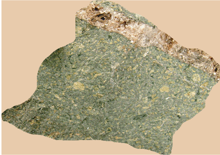
Figure 3. Propylitic altered (unit pr) Burns Member of the Silverton Volcanic Series lavas. Plagioclase phenocrysts (light-green, tabular to equant grains) have been altered to a mixture of chlorite and epidote and minor sericite. Darker green groundmass is also altered to a mixture of same constituents. Sample about 4.5 cm across.
