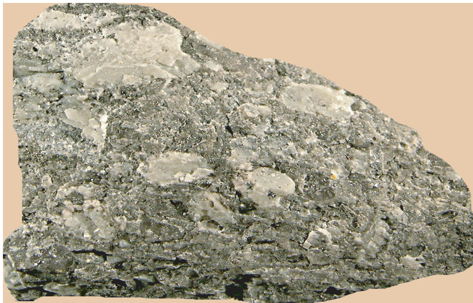
Figure 10. High-level, argillic altered dacite porphyry intrusive rock. Relict feldspar phenocrysts have been replaced by white, waxy, dickite. Dickite is soft and easily scratched with a fingernail. Sample 5 cm wide.
