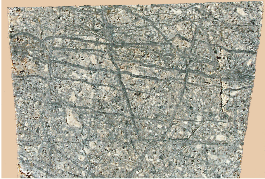
Figure 5. Quartz-sericite-pyrite (unit qsp) altered quartz monzonite intrusive with dense stockwork quartz veinlets. Sample from 1 km 2 area of unit qsp alteration centered around peak 3,792 m (informally referred to as Mount Moly) (fig. 1) due to nearby molybdenum exploration. Stockwork veinlet densities are anomalously high (0.3–1.5/m 2 ) in this area of intense alteration; note offset in veinlets. Slab nearly 9 cm across.
