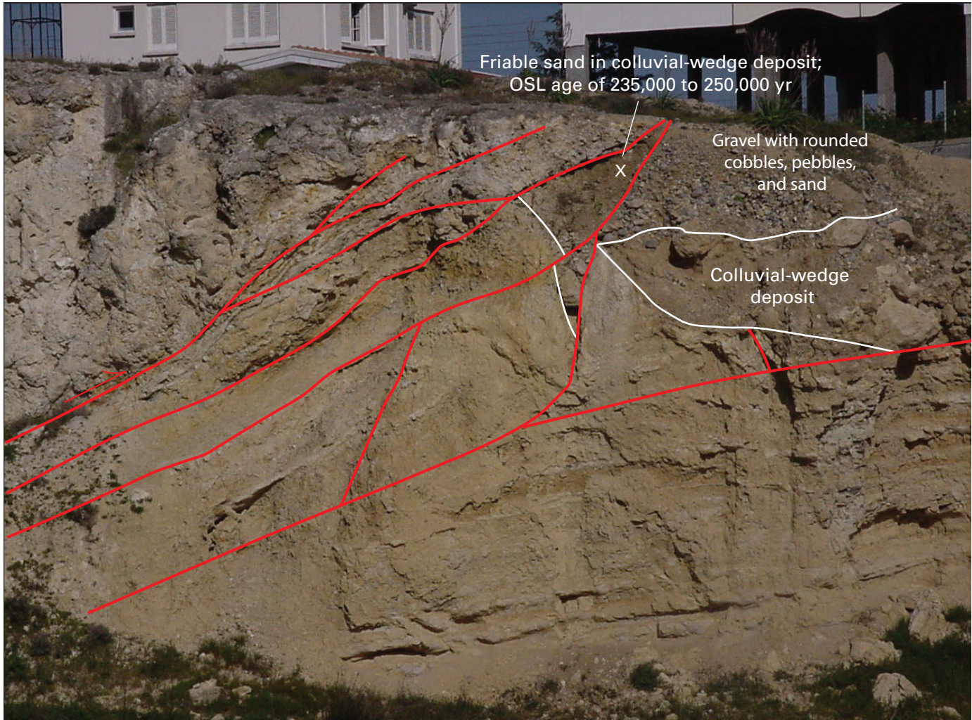
Figure 22. View of the northeastern part of the positive flower structure on the Skali fault showing low-angle thrust faults and relations of calcified breccia, colluvial-wedge, and Quaternary alluvial deposits. OSL, optically stimulated luminescence.
