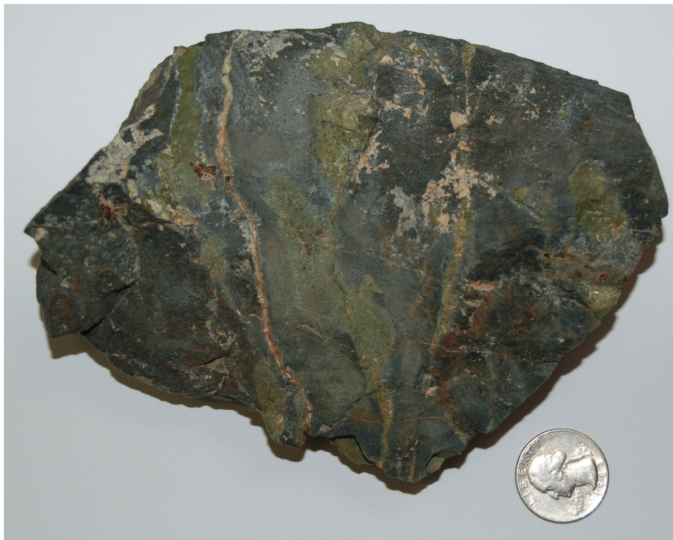
Figure 1. Propylitically-altered metavolcanic rock from the Excelsior Formation in the Wassuk Range southwest of Hawthorne, Nev. Note green chlorite and epidote. Sample WSK09-1 collected at 118.689513 W., 38.449715 N. (WGS 84).
