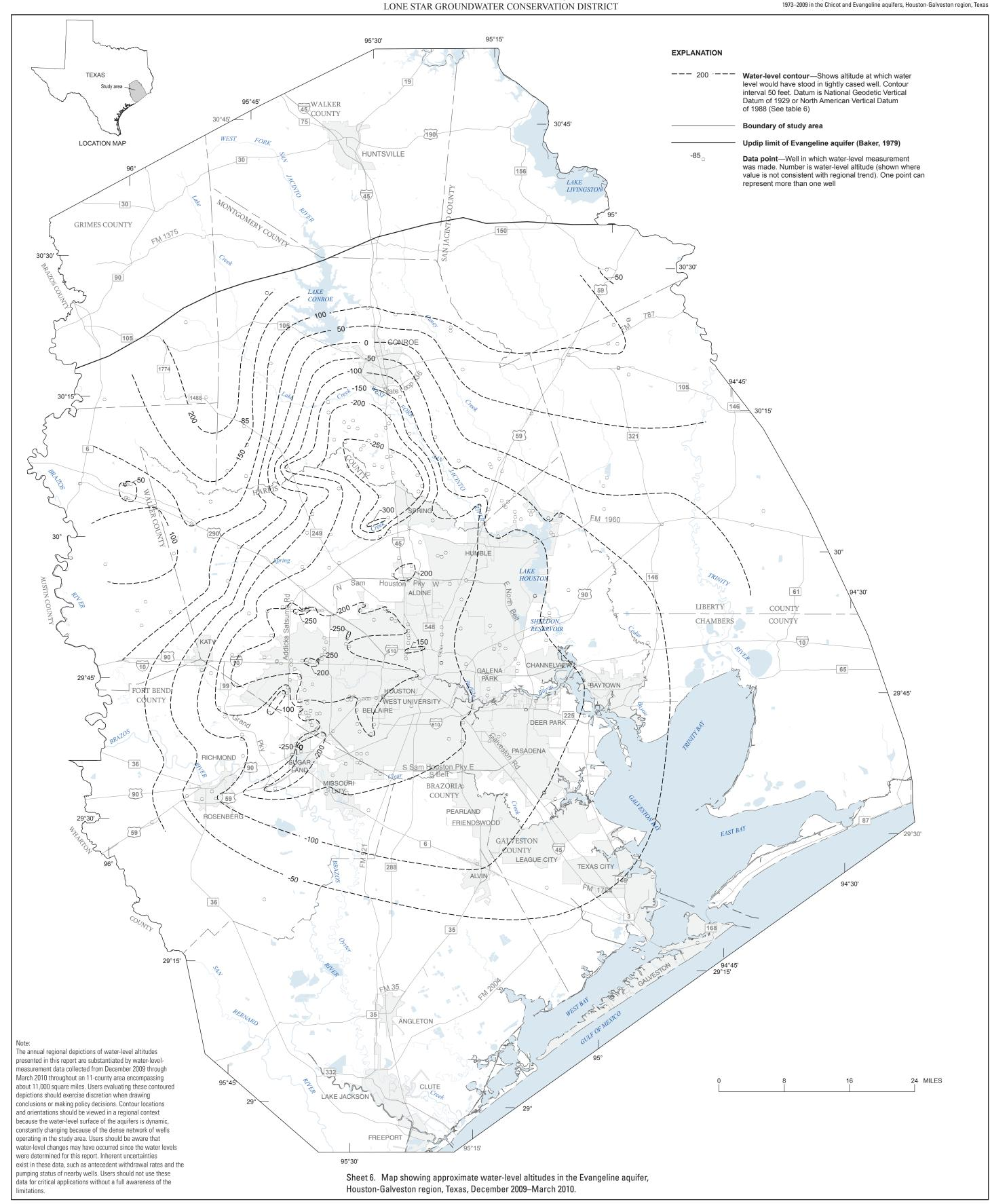
Base from U.S. Geological Survey digital data, 1:100,000 Universal Transverse Mercator projection, zone 15 North American Datum of 1927 Water-Level Altitudes 2010 and Water-Level Changes in the Chicot, Evangeline, and Jasper Aquifers and Compaction 1973–2009 in the Chicot and Evangeline Aquifers, Houston-Galveston Region, Texas
