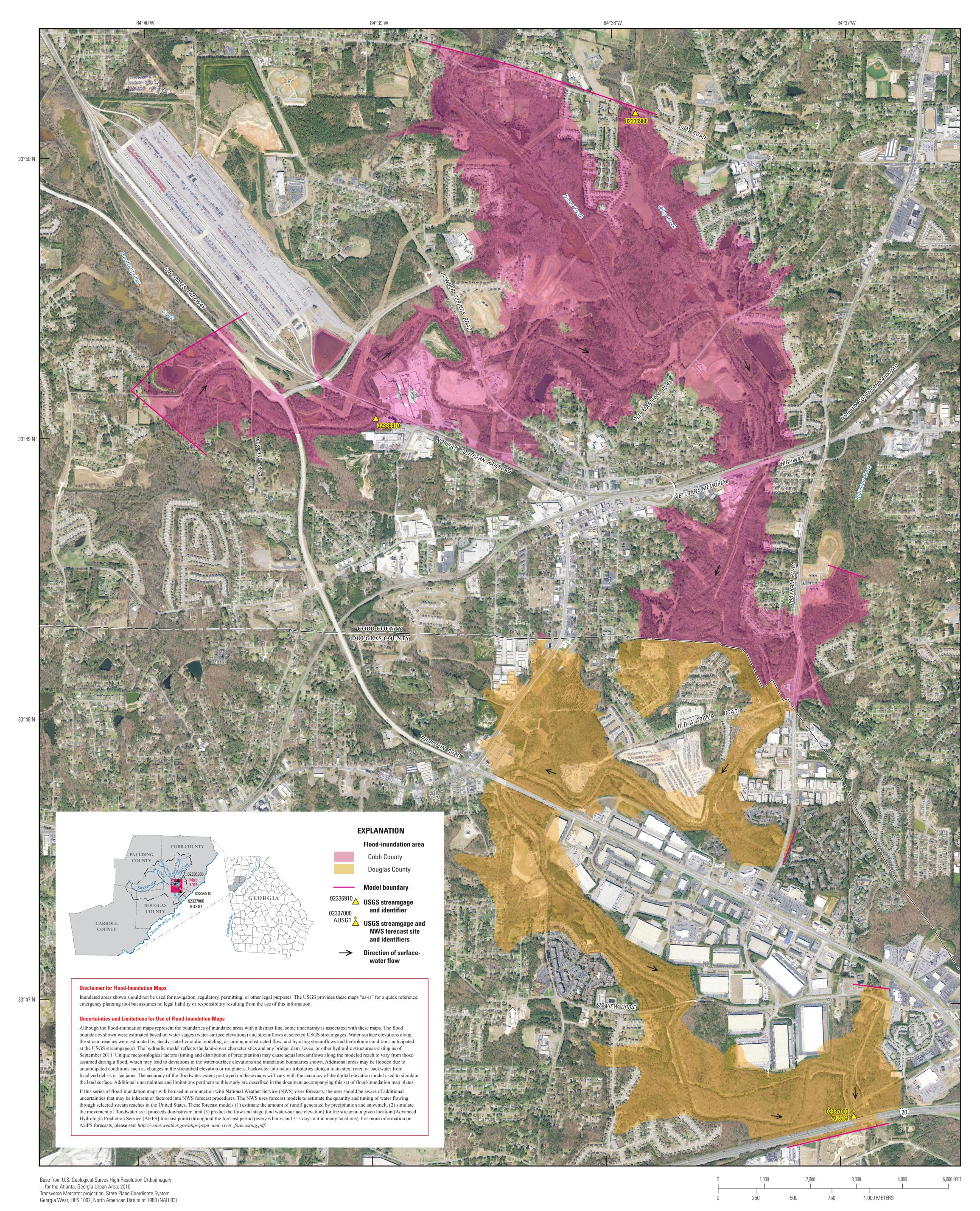
Flood-Inundation Map of Sweetwater Creek in Cobb and Douglas Counties, Georgia, Corresponding to a Gage Height of 29.0 Feet and an Elevation of 886.3 Feet (NAVD 88) at the U.S. Geological Survey Streamgage Sweetwater Creek near Austell, Georgia (Station ID 02337000)
