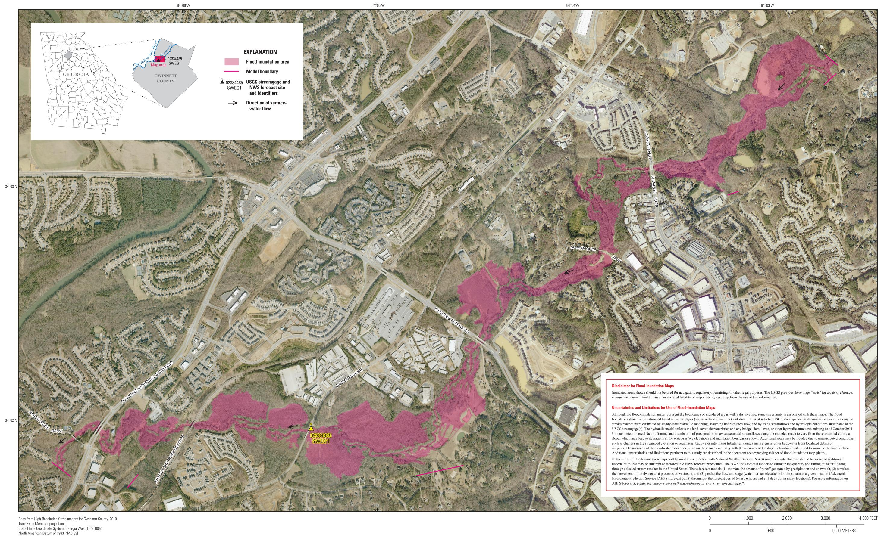
Flood-Inundation Map of Suwanee Creek in Gwinnett County, GA, Corresponding to a Gage Height of 8.0 Feet and an Elevation of 917.9 Feet (NAVD 88) at U.S. Geological Survey Streamgage Suwanee Creek at Suwanee, GA (02334885)
