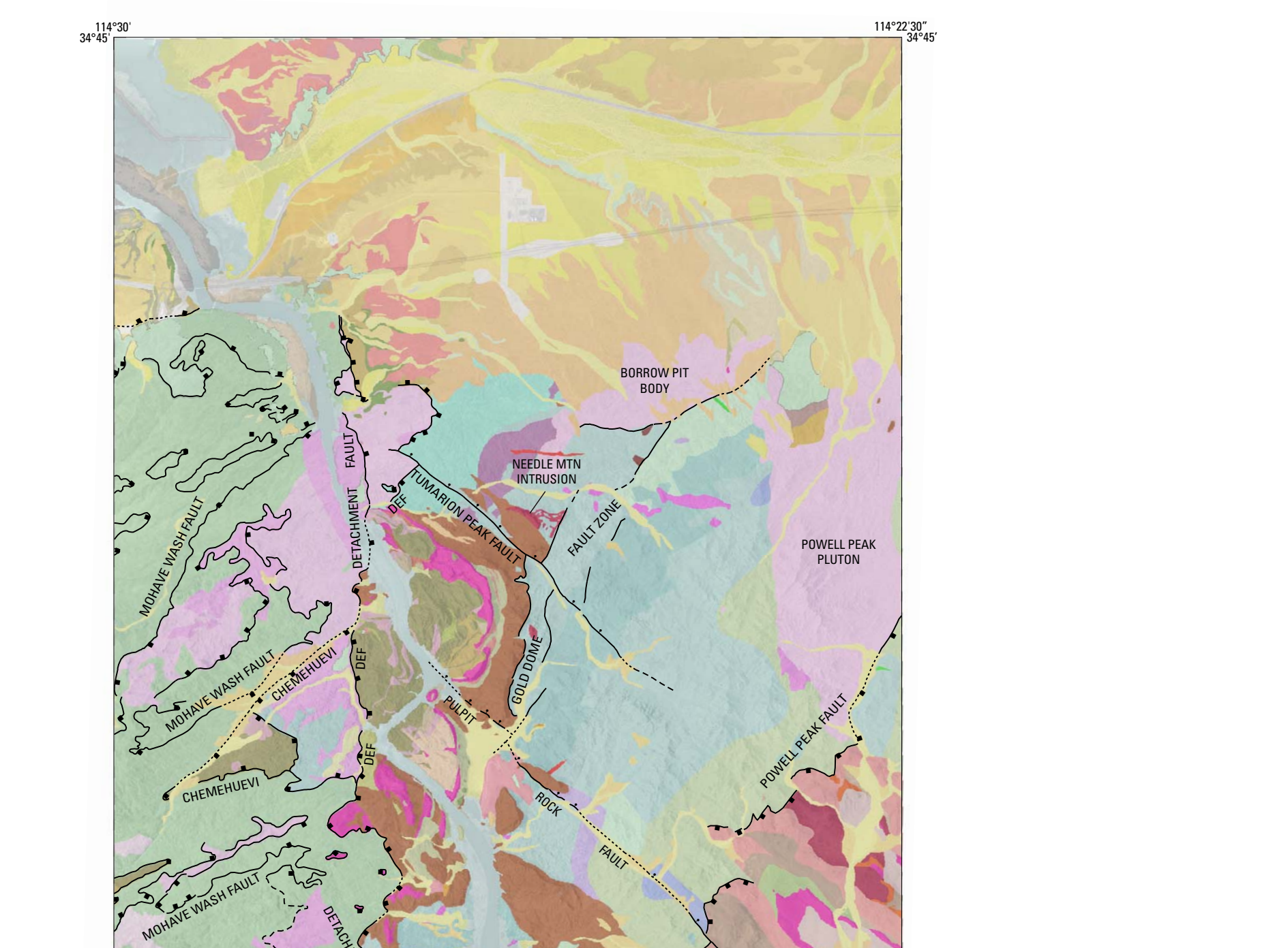
Figure 2. Map showing Topock quadrangle geology and major structures draped over hillshade derived from 30-meter digital elevation model. Devil's Elbow Fault (DEF).
