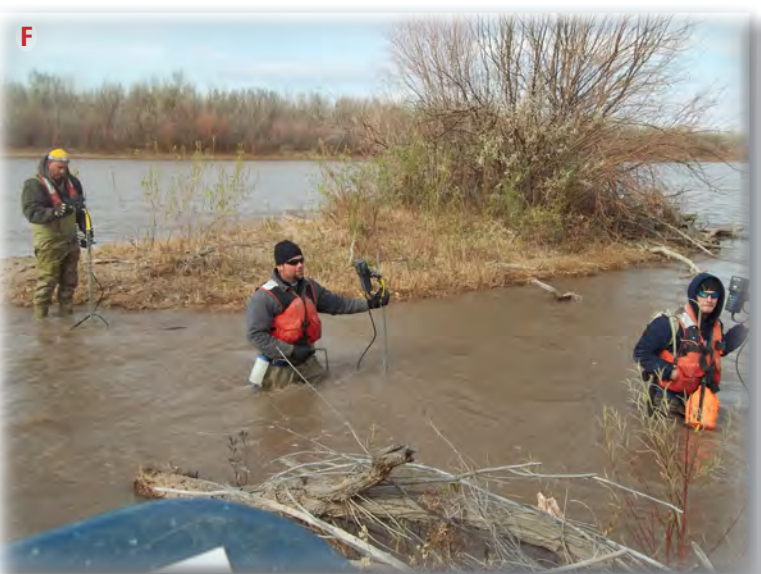
Measuring depths and velocities in a run (mesohabitat ID 10). Photograph by Daniel K. Pearson, U.S. Geological Survey, December 2, 2011.
