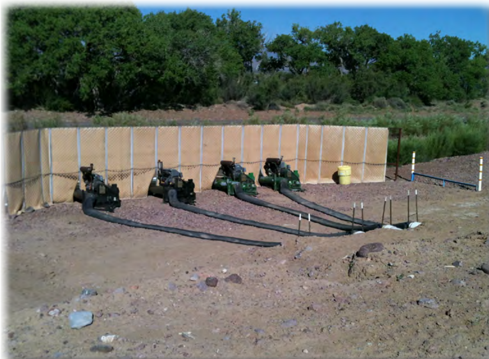
Pumps transferring water from the conveyance channel to the main channel of the Rio Grande near San Pedro; the photograph was taken outside the mapped area shown. Photograph by Daniel K. Pearson, U.S. Geological Survey, June 9, 2012.
