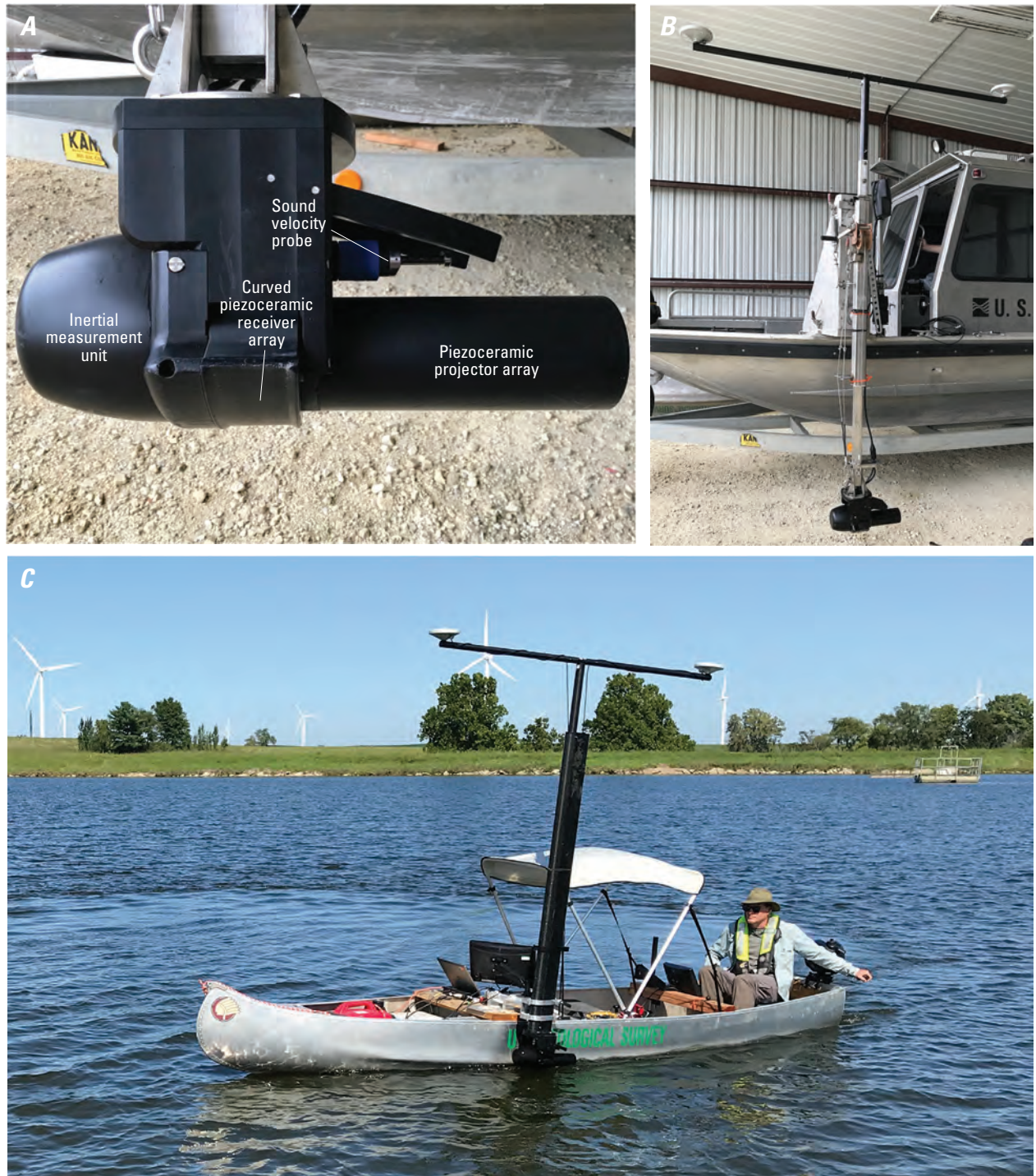
Figure 2. The Norbit iWBMSH multibeam echosounder. A , Viewed from the side. B , Mounted on the port side of the U.S. Geological Survey 22-foot cabin boat. C , Deployed on the port side of the 18-foot cargo canoe.
