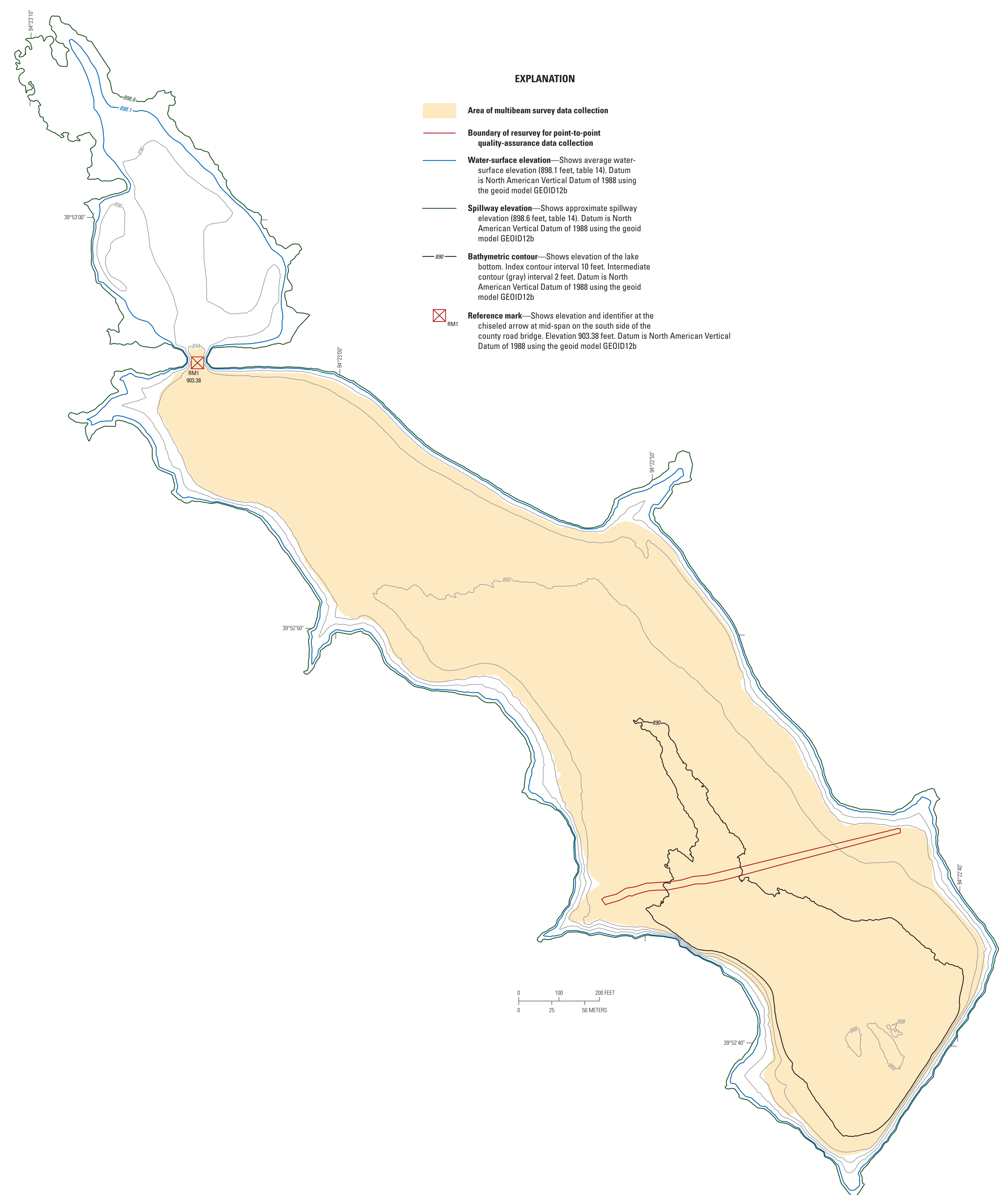
Figure 45. Bathymetric contours for Maysville Reservoir (lake 10; fig. 1; table 1) near Maysville, Missouri, resulting from a survey on September 7, 2019.
