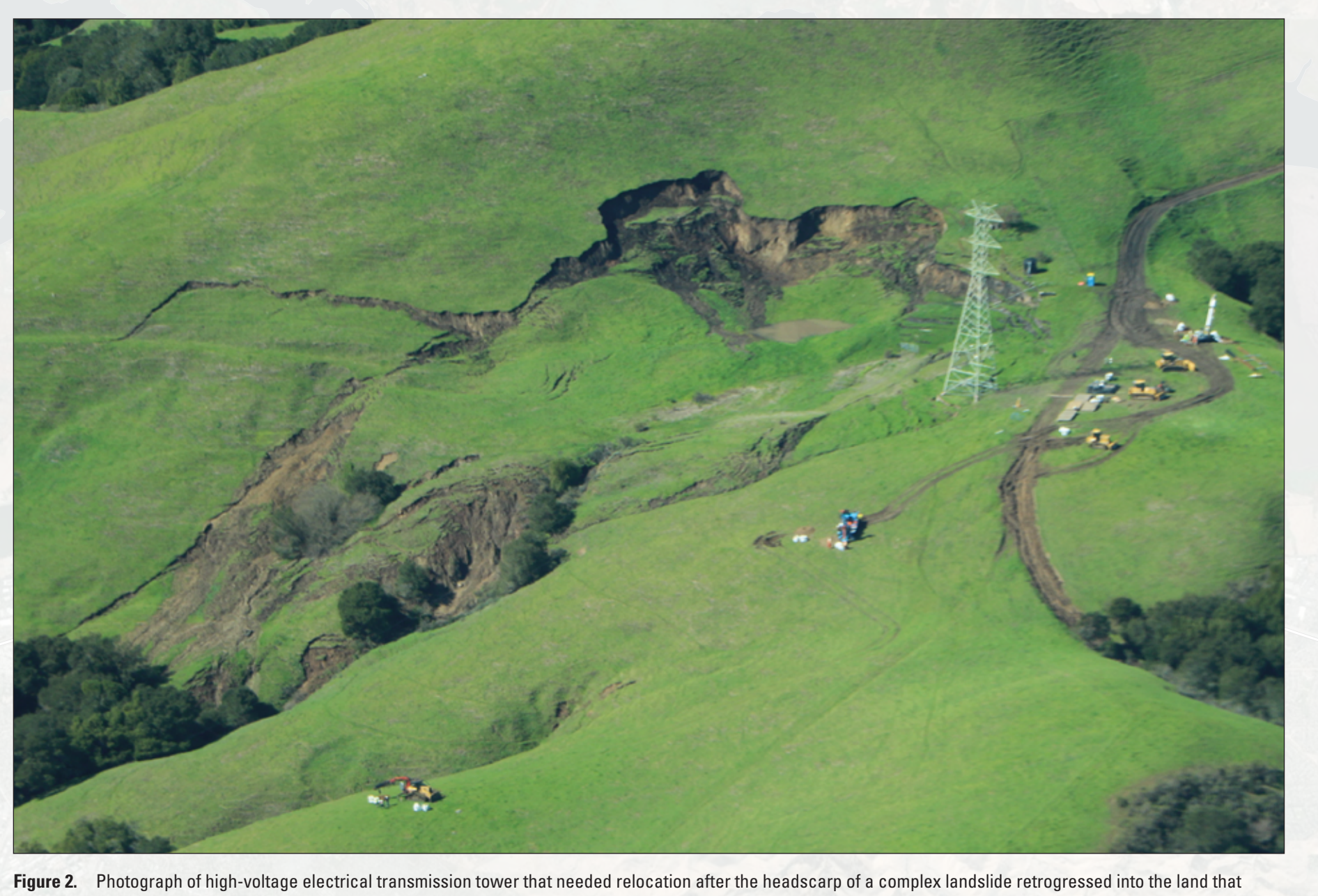
Figure 2. Photograph of high-voltage electrical transmission tower that needed relocation after the headscarp of a complex landslide retrogressed into the land that supported its foundation during the storms of early 2017. See main map image for location. Photograph taken February 23, 2017.
