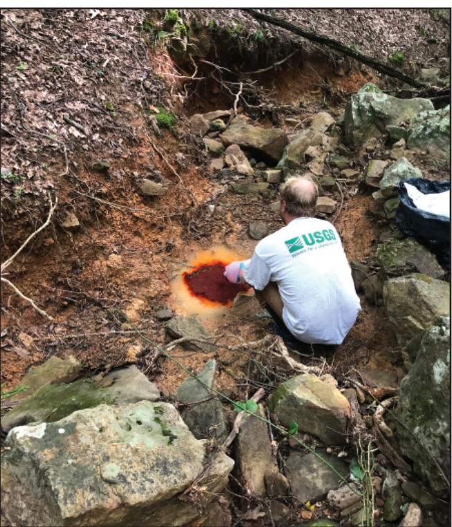
Figure 6. Injection of fluorescent dye at injection site I-10, July 28, 2020. Photograph by Ben Miller, U.S. Geological Survey.
