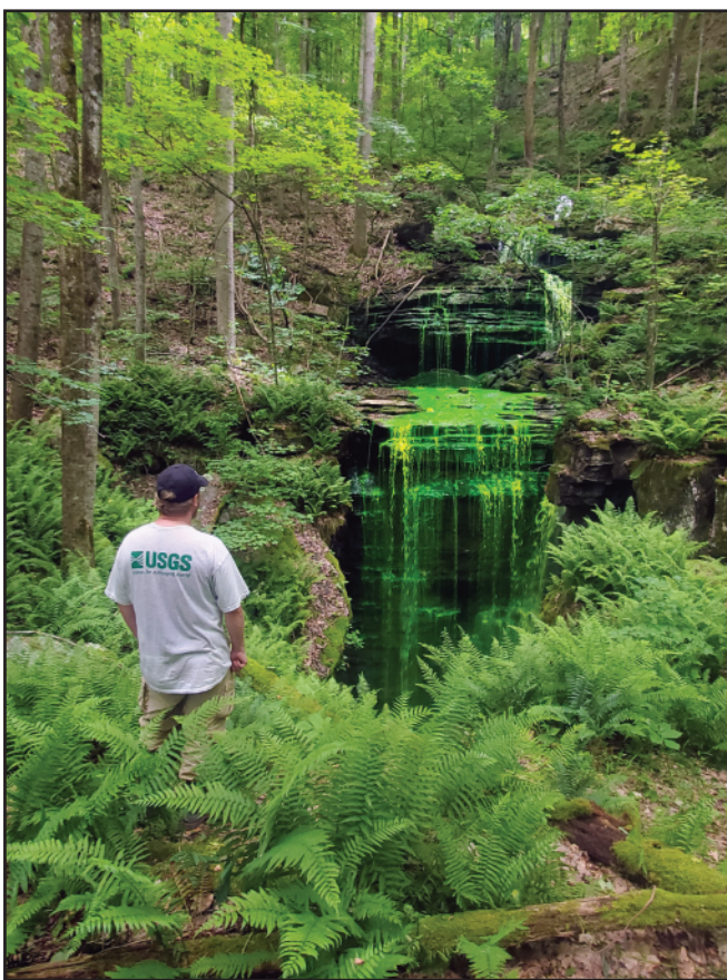
Figure 8. Injection of fluorescein dye into Surprise Karst Window (injection site I-13), May 18, 2021. U.S. Geological Survey (USGS) scientists followed all appropriate safety protocols and requirements for working near, on, in, or over water consistent with approved USGS Job Hazard Analysis. Photograph by Ben Miller, U.S. Geological Survey.
