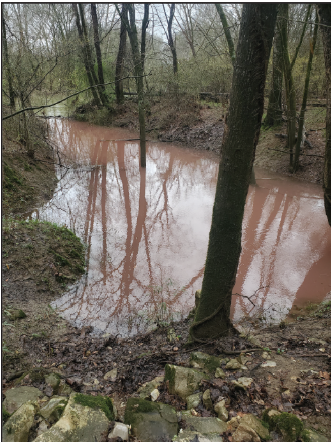
Figure 5. Visual confirmation of eosine dye and sulfolhodamine B determined via chemical packets at Haley Spring (monitoring site 001), March 15, 2020. Photograph by Ben Miller, U.S. Geological Survey.
