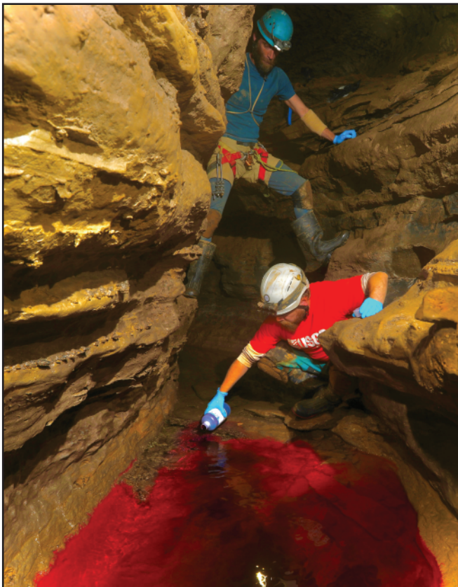
Figure 7. In-cave dye injection of rhodamine WT into Lower North Cave Stream (injection site I-12), May 18, 2021. U.S. Geological Survey (USGS) scientists followed all appropriate safety protocols and requirements for working near, on, in, or over water consistent with approved USGS Job Hazard Analysis. Photograph by Brian Ham, used with permission.
