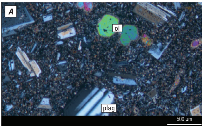
Figure 4.64. Thin-section photographs of sample of lava flow from Pavlof Volcano (unit plh), in Emmons Lake volcanic center, Alaska. A , Photograph 02S53M1-1, in cross-polarized light. B , Photograph 02S53M1-2, same view as A but in plane-polarized light. Abbreviations: μm, micrometer; ol, olivine; plag, plagioclase.
