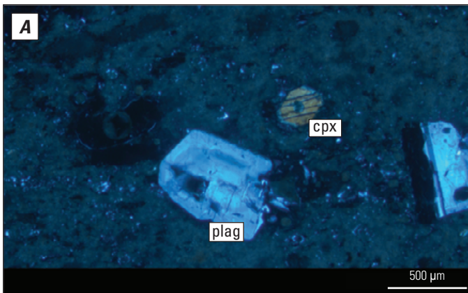
Figure 4.54. Thin-section photographs of sample of pumiceous pyroclastic-flow deposit (unit pfd), in Emmons Lake volcanic center, Alaska. A , Photograph 99S1M1-1, in cross-polarized light. B , Photograph 99S1M1-2, same view as A but in plane-polarized light. Abbreviations: \mu\text{m} , micrometer; cpx, clinopyroxene; plag, plagioclase.
