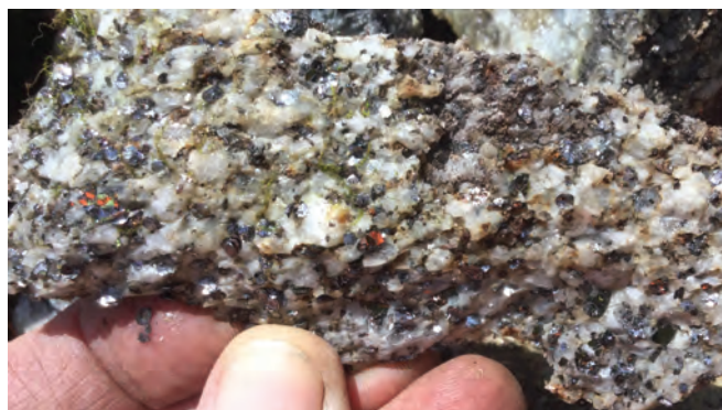
Figure 23. Photograph of flake graphite in marble at the Crown Point Graphite Company deposit; location: 43.894544, -73.572131 (WGS 84). Photograph by Gregory J. Walsh, U.S. Geological Survey.
