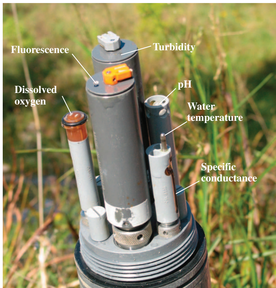
Figure 2. Multiparameter monitor used to measure specific conductance, pH, water temperature, turbidity, dissolved oxygen, and fluorescence in water during sample collection and for in-stream and in-lake continuous monitoring.
