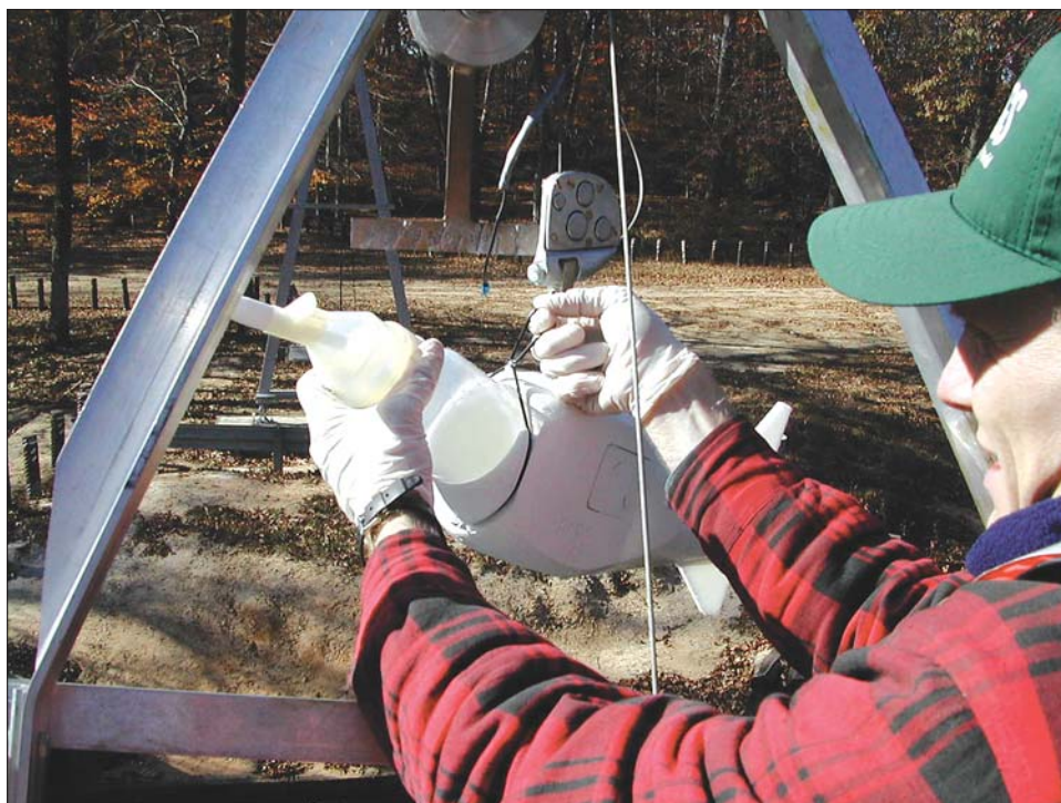
Figure 5. DH-95 isokinetic sampler with 1-liter Teflon bottle. (Photograph by Michael P. Senus, U.S. Geological Survey)
