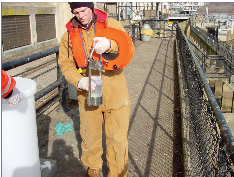
Figure 4. Stainless-steel weighted-bottle sampler and hand-reel with polyethylene rope. (Photograph by Michael P. Senus, U.S. Geological Survey)
