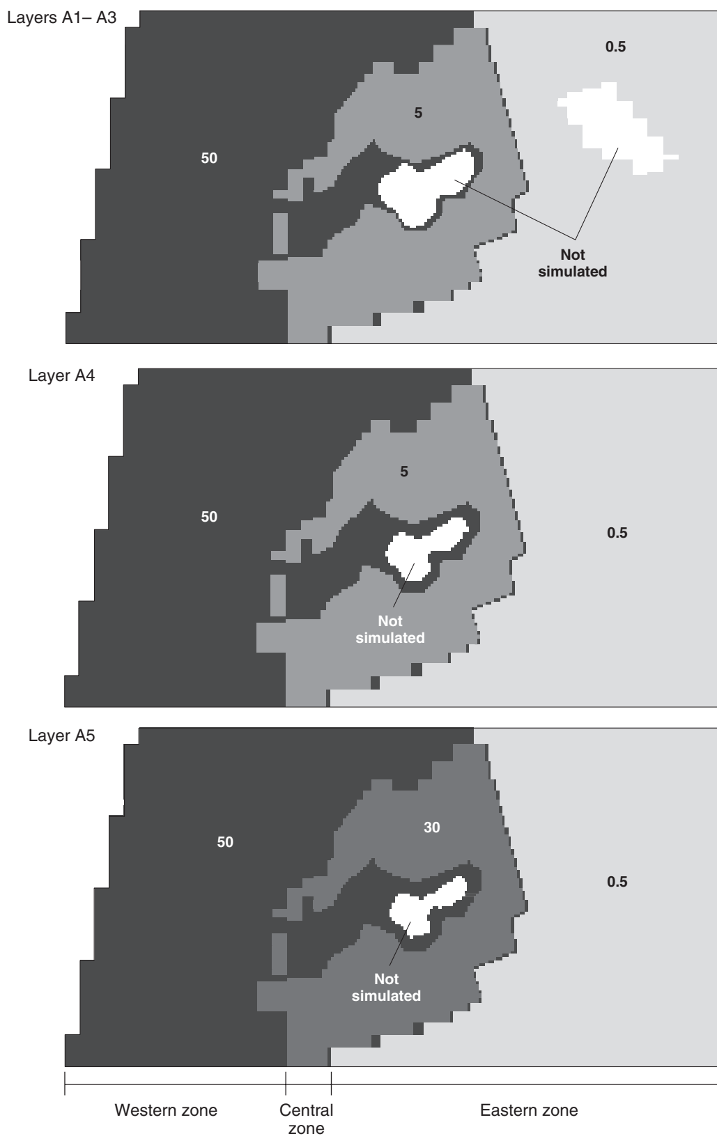
Figure A8. Simulated horizontal hydraulic conductivity in feet per day in model layers A1 through A5 at the Glynn County pond site in Georgia.
