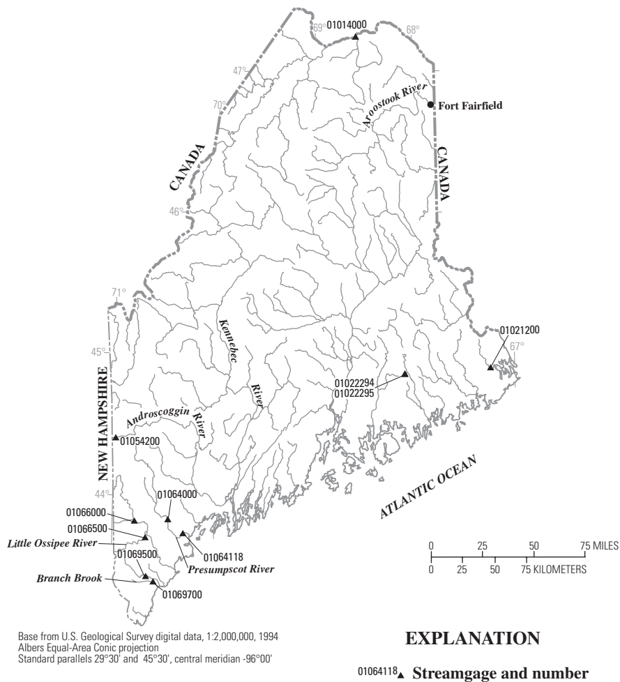
Figure 31. Location of streamgages with significant floods during 1994–98 water years for Maine.
