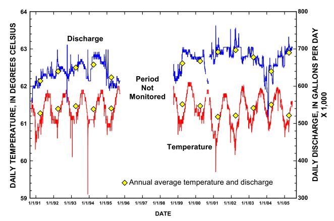
Figure 7. Daily and annual average discharge and temperature of the thermal springs at the inflow of the collection system reservoir.
