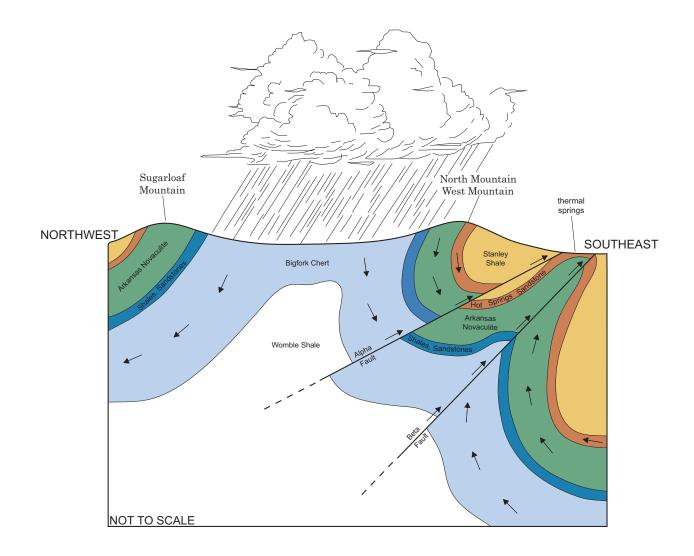
Figure 13. Conceptual model of the thermal water flow system.
