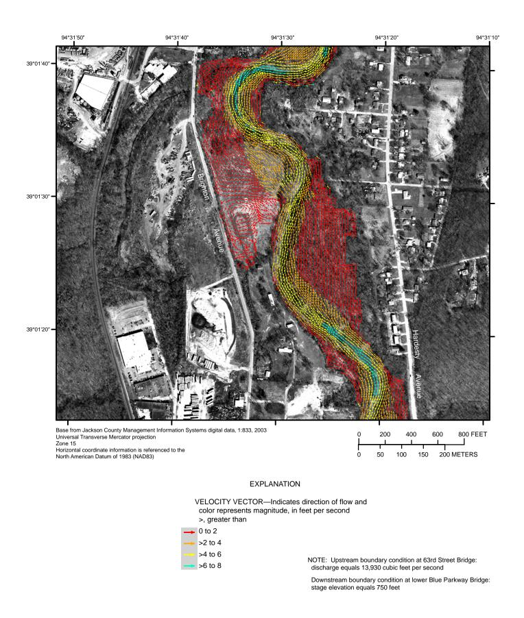
Figure 2.1. Two-dimensional model results depicting velocity magnitude and direction between 63rd Street and Blue Parkway.
