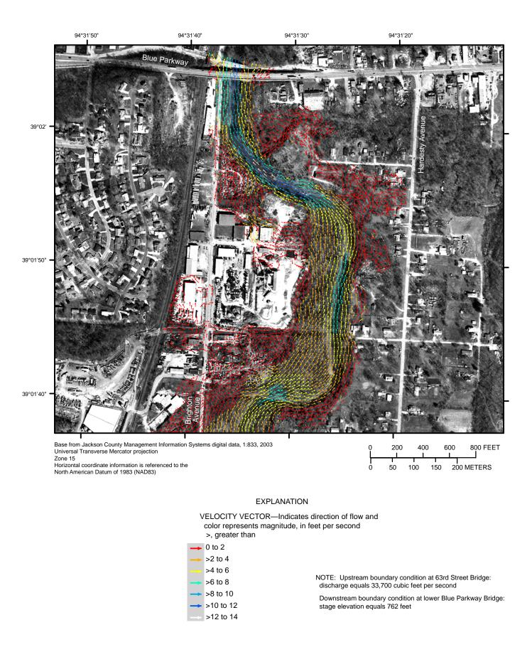
Figure 3.7. Two-dimensional model results depicting velocity magnitude and direction in the upstream vicinity of Blue Parkway.
