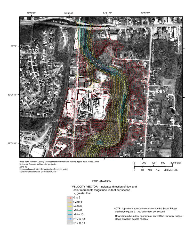
Figure 3.8. Two-dimensional model results depicting velocity magnitude and direction in the upstream vicinity of Blue Parkway.
