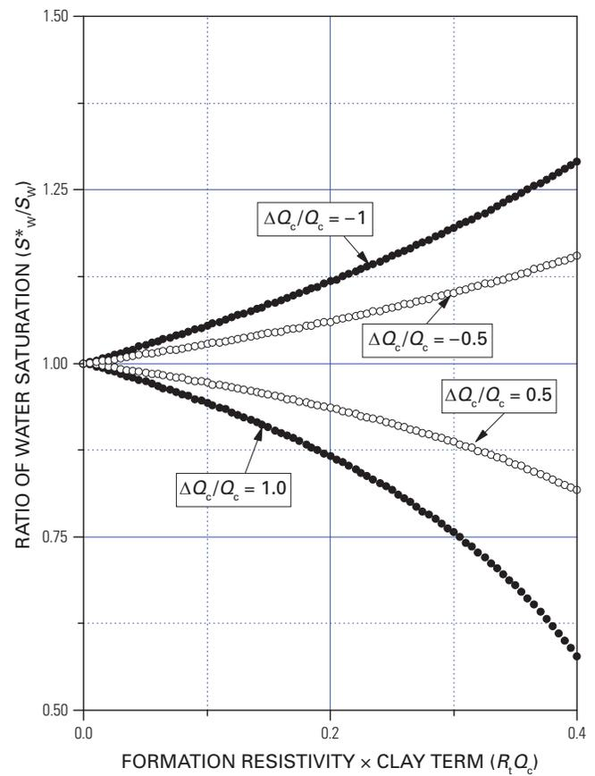
**Figure 8.** Graph showing the ratio of water saturation versus the formation resistivity times the clay term ( $R_{tQ_c}$ ) for different relative errors in the clay term ( $Q_c$ ).  $S_w$  is the water saturation estimated from the resistivity when there is no error in  $Q_c$ , and  $S_w^*$  is the estimated water saturation when there is a relative error in  $Q_c$ . Solid dots indicate an error of 100 percent, and open circles are errors of 50 percent.
