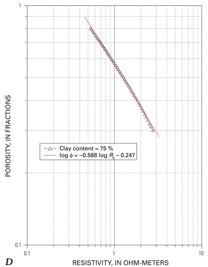
**Figure 2 (previous page).** Plots of logarithm of the porosity versus logarithm of the resistivity to show the linear relationship. The model parameters are identical to those for figure 1A, which are  $a = 1$ ,  $m = 2$ , water resistivity ( $R_w$ ) = 0.35  $\Omega$ -m, and clay resistivity ( $R_c$ ) = 5  $\Omega$ -m. Plots are for A, clean sand; B, 25 percent clay; C, 50 percent clay; and D, 75 percent clay.
