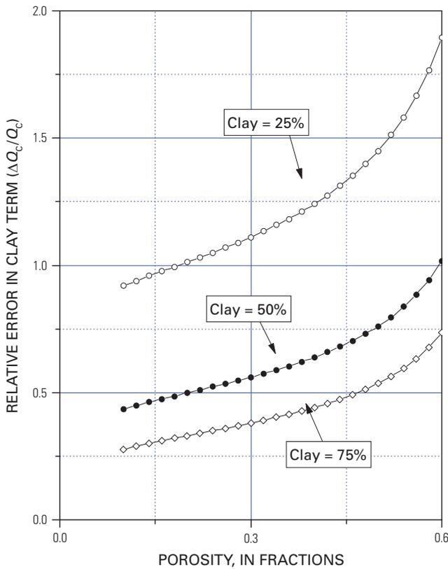
**Figure 7.** Graph showing relative errors in estimating the conductivity contributed by clay versus porosity. The parameters for various clay contents are identical to those for figure 1A, and the error in  $m$ ,  $\Delta\mu$ , is 0.1.
