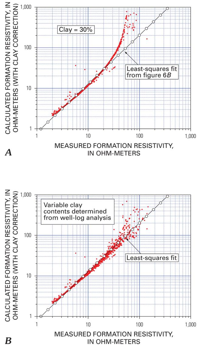
**Figure 6.** Plots showing clay-corrected resistivity versus observed resistivity at the Mallik 2L-38 well, Mackenzie Delta, Canada. Archie constants for shaly sand are  $a^* = 1.02$  and  $m^* = 1.95$ , and for a clean sand they are  $a = 1$  and  $m = 2$ . The resistivity of connate water was set to  $0.25 \Omega\text{-m}$ . *A*, Using constant clay contents (average of 30 percent). *B*, Using variable clay contents from well-log analysis.
